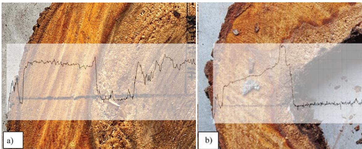
Figure 1. Rinntech RESISTOGRAPH® R650 drilling profile and actual cross-cut at corresponding height:
