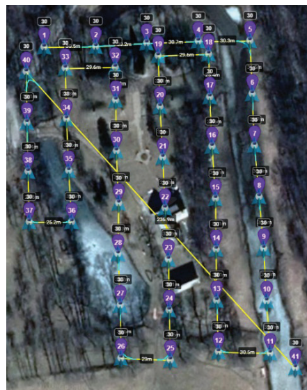
Figure 9. UAV flight routes executed over territory of museum: mission hub – Litchi for DJI Mavic, version 2.9.1.
