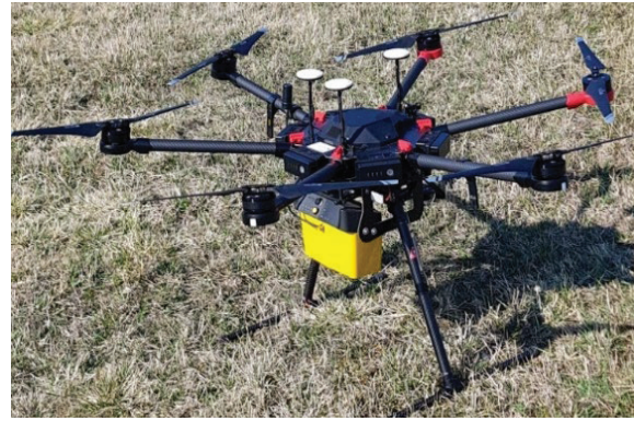
Figure 2. UAV with equipped gimbal camera, laser scanner, GPNS used for photogrammetric data collection of study area.
