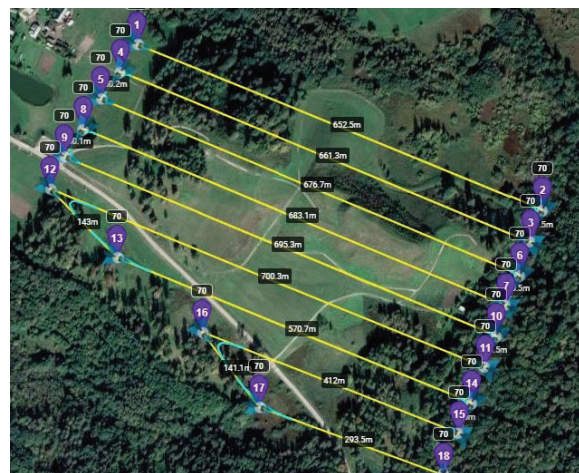
Figure 3. UAV flight mission: flight strips over experimental area.
