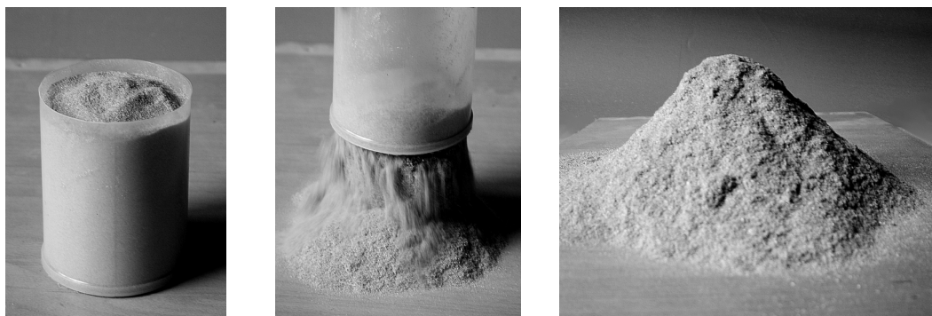
Fig. 2. Obtaining of the angle of repose.
