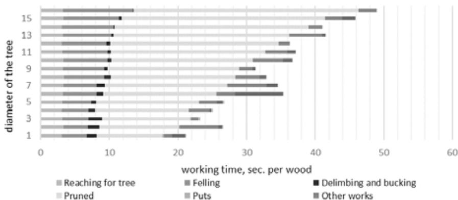
Figure 4. Distribution of work time consumed (sec. per processing of a single trunk) in different diameter classes in young coniferous stands.
